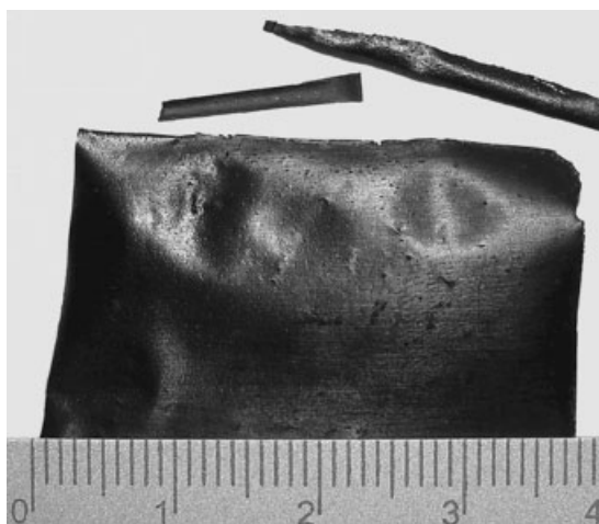
Figure 10 Photograph of free-standing poly(Th-co-DOF = 1 : 1) films electrodeposited on the electrode surface from 80% BFEE containing 20% EE solution at a constant applied potential of 1.55 V vs. SCE.
